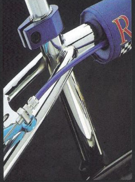
Alloy seat mast clamp with allen bolt
