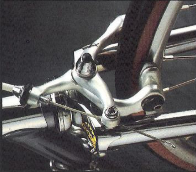
Aero alloy sidepull brakes with drilled levers and gum hoods
