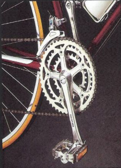
Triple alloy crank set with alloy platform pedals
