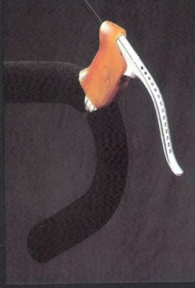
Alloy sidepull brakes with drilled levers and gum hoods
