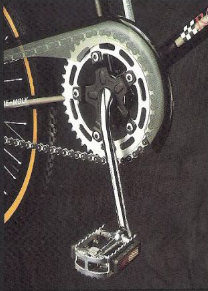
Chrome moly crank spider and alloy chain ring
