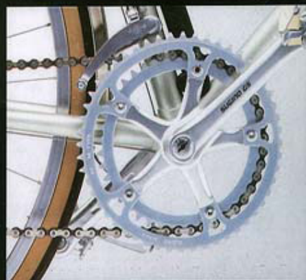
Sugino GS long arm fully detachable chainwheel
