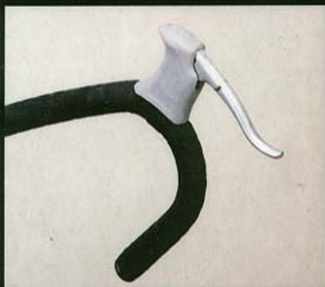
Shimano Adams hooded levers with concealed cables
